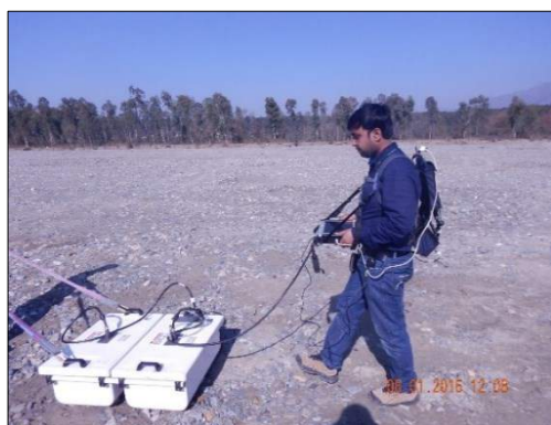
Figure 22 GPR Data acquisition using 100 MHz
