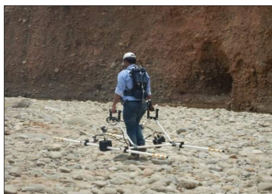
Figure 21 GPR Data acquisition using 40 MHz
