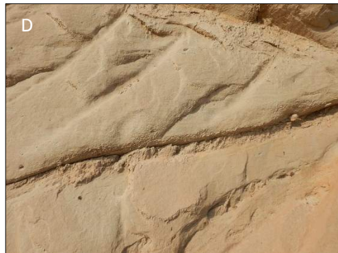
Above figure shows (A) Strike slip movement of bed (B) Slickensides (C) Triangular facets near fault plane and (D) Intrusion of clay layer in the fault plane.
