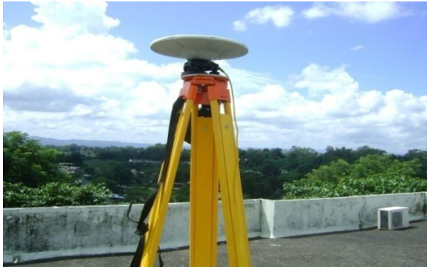
Figure 5.6 GPS base receiver at roof top
