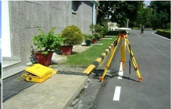
Figure 5.7 GPS rover receiver in front of the buildings
