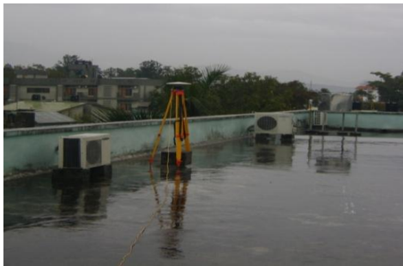
Figure 4.10 GPS observations on Wet surface
