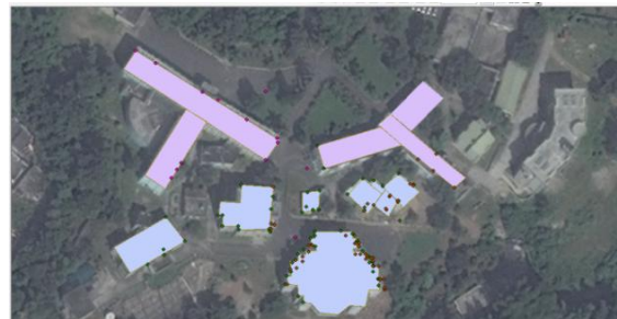
Figure 3.7 Creation of shapefile using footprints
