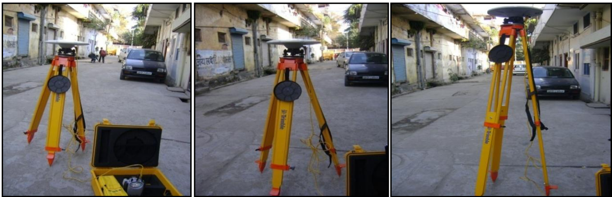
(a) Antenna Height 1 m (b) Antenna Height 1.4 m (c) Antenna Height 1.8 m
