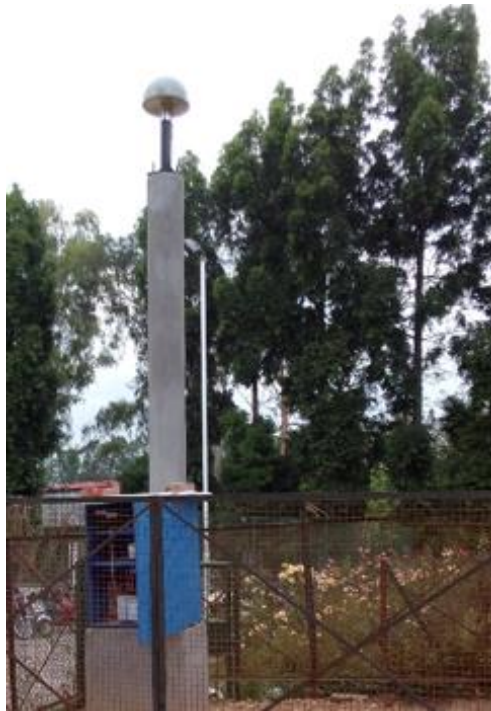
Fig. 3.10 CORS Stations established at IIRS Campus showing NetR9 receiver at the top of tower with an antenna Radome. Housing for other instrumentation and accessories is visible at the bottom
