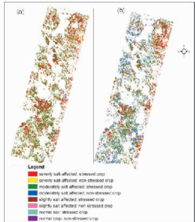
Soil salinity mapping (a) Modified Red Edge NDVI (b) Structure Intensive Pigment Index
