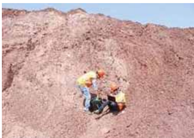
Spectra collection in field from Joda Mines, Odisha and Matun Mines, Rajasthan using ASD Field Spec4 Spectro-radiometer (0.5-2.5 micro meters).
